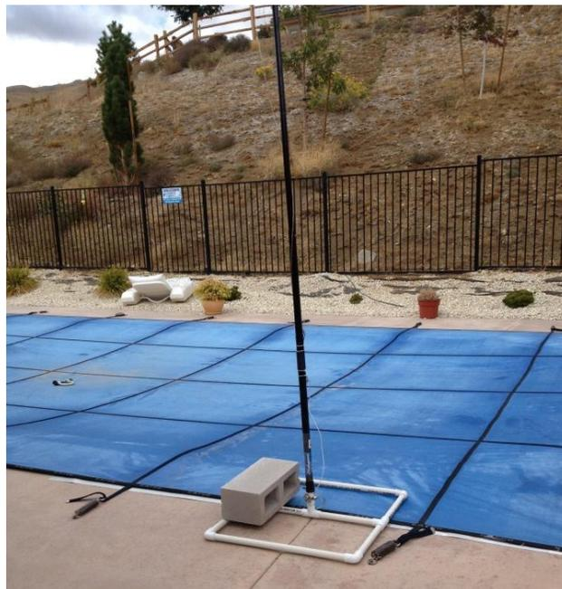
**The Wonderpole 40 meter vertical, efficient but non-stealthy, useful only at night. Barely visible under the pool cover is a 10 ft X 12 inch aluminum ground plate.**
