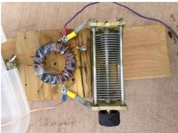
**The tuned circuit for the end-fed half wave antenna. An Amidon FT240-43 toroid core has primary and secondary inductances. A dual section 200 pF capacitor (sections in series) handles the tuning. The purple wire is the 3 ft "counterpoise". This circuit sits at ground level, and is normally covered to keep out rain and snow.**
