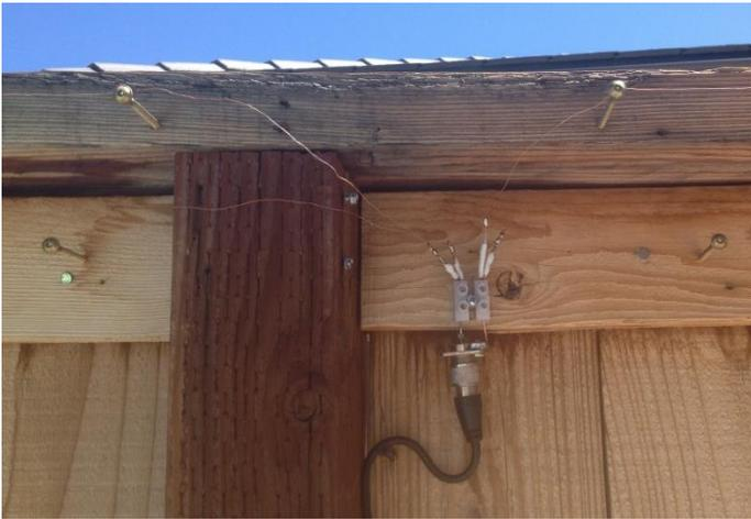
Center of a 20/15 meter dual dipole on a 6 ft high fence, using vinyl window screws for wire support. A Euro-block from Radio Shack makes for easy connections.
